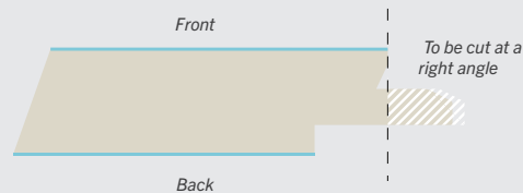
Diagram 2: Cutting off the male part (tongue)
